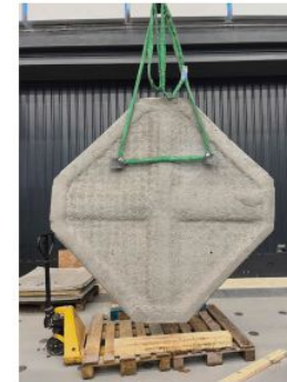
(a) Central segment with 2.5 m long ribs
