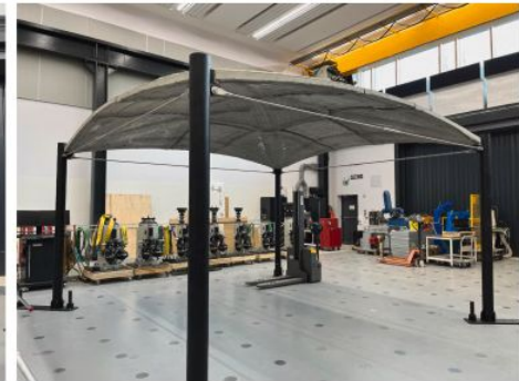
(b) Assembled nine segment shell demonstrator on columns
